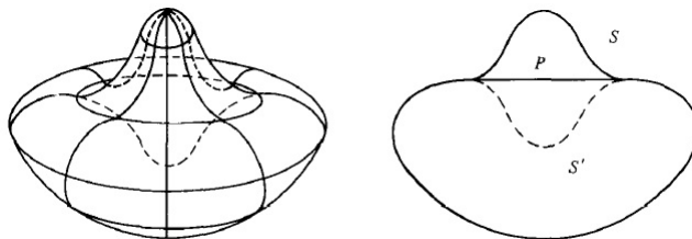
Figure 2: Surfaces that are homeomorphic to a sphere and that are not rigid.
