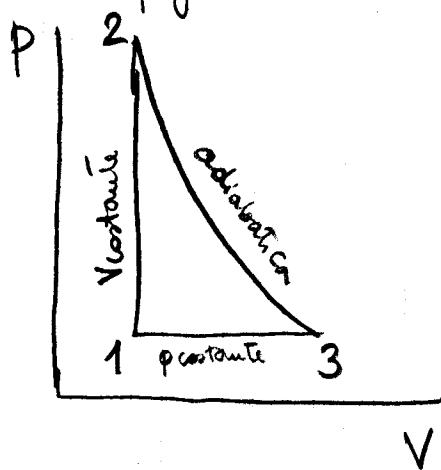
$$\begin{aligned} T_1 &= 300 \text{ K} \\ p_1 &= 1,0 \text{ atm} \\ T_2 &= 600 \text{ K} \end{aligned}$$
